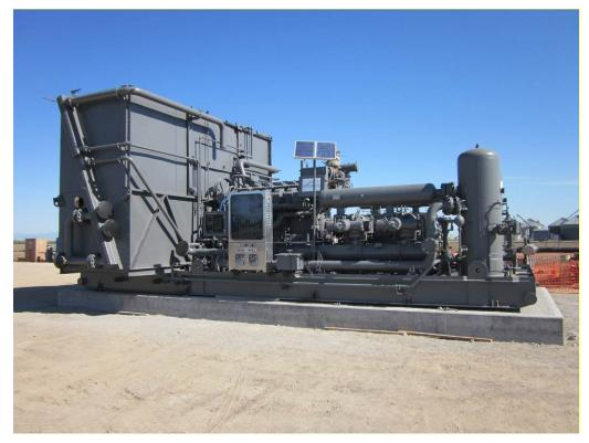
**Photo 2:** Temporary compressor placed at the remote well pad site.
